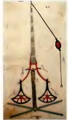
A traction trebuchet for hurling missiles from a 14 th -century Manual on Armoury by Ibn Aranbugha al-Zardkash.
